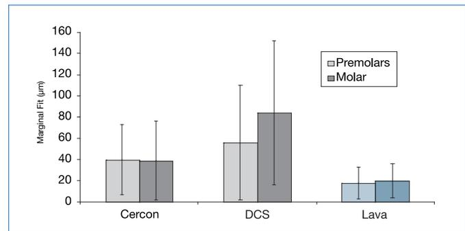
**fig. 2a** Marginal gap of 4-unit zirconia 3M™ ESPE™ Lava™ Bridges in comparison to competitor systems. A. Piwowarczyk and H.C. Lauer, University of Frankfurt.<sup>2</sup>
