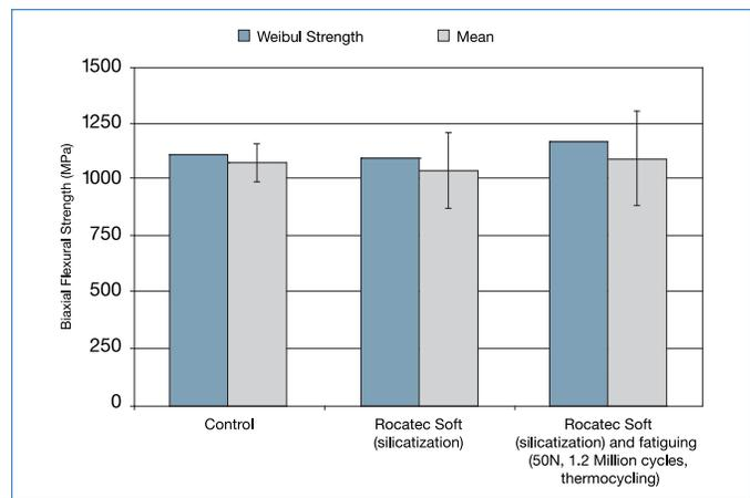
fig. 3 No strength reduction after 3M™ ESPE™ Rocatec™ Soft Treatment (30μm) of 3M™ ESPE™ Lava™ Zirconia initially and after cyclic loading and thermocycling (50N, 1.2 Million cycles).
