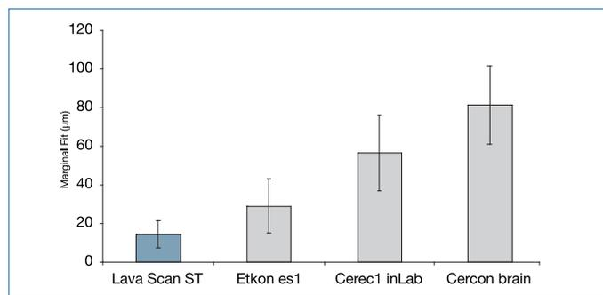
**fig. 3** Marginal gap of 3-unit zirconia 3M™ ESPE™ Lava™ Bridges in comparison to competitor systems. F. Beuer et al., University of Munich.<sup>3</sup>
