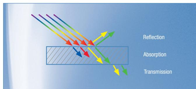
**fig. 2** Example of reflected an transmitted light versus absorbed light. The observer detects light of the remaining wavelength, in this case green and yellow light.
