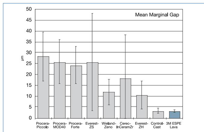
**fig. 4** Vertical marginal gap of 3M™ ESPE™ Lava™ Copings in comparison to competitor systems. A.J.T. Shannon et al., University of Iowa.<sup>4</sup>
